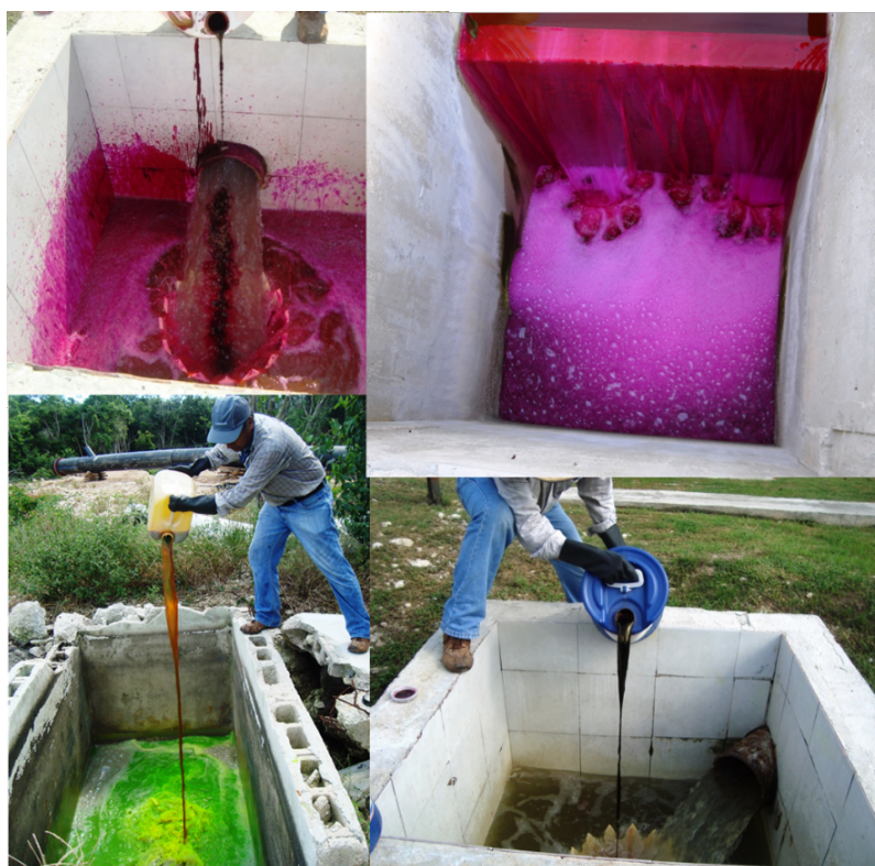
FIGURE 3. Application of Rhodamine WT and Fluorescein. Source: own elaboration.
