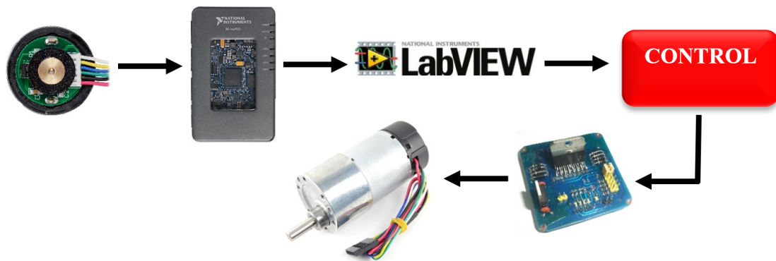
FIGURA 4. The electronic scheme applied to sensing and control.
